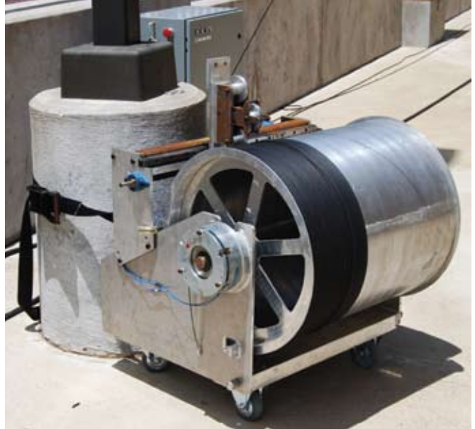
Spring applied brakes from Ogura are used to hold the control cables of ActionCam overhead stadium cameras, high definition cameras used in football stadiums and other sporting venues.
