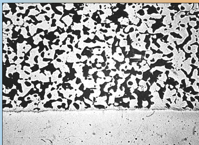
Figure 3 — Real bearing alloy microstructures. Type I: lead-base babbitt. Dark phase — Pb, light phase — Sb. Type II: copper-lead. Dark phase — Pb, light phase — Cu. Type III: medium-lead tin bronze. Dark phase — Pb, light phase — Cu-Sn. Original magnification 100 \times . Courtesy, Glacier Vandervell Inc.
