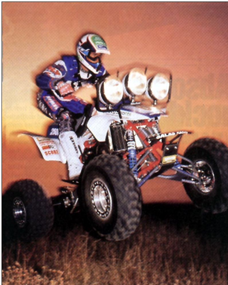
Racing-type all-terrain vehicle about to come down hard on its shock absorbers. Injection-molded thermoplastic plain linear bearings inside the custom-made shocks and similar bearings in the eye mounts keep shocks at peak performance even during the toughest of rides.
