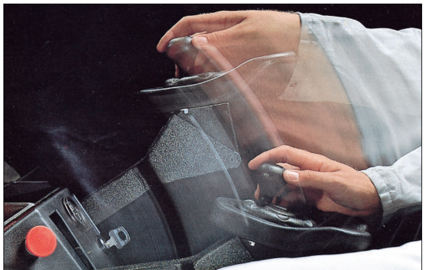
Figure 3 — Operator's steering control can be placed in the most convenient location for the operator, because only two control wires connect the operator's control to the steering controller. As shown here, the "steering wheel" is mounted on a tiltable arm. (Photo courtesy of BT Products AB.)
