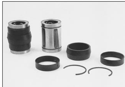
Conventional steel linear bearing with resilient mount. Assembled unit on left. This approach not recommended for use with self-aligning bearings. Courtesy, Thomson Industries Inc.
